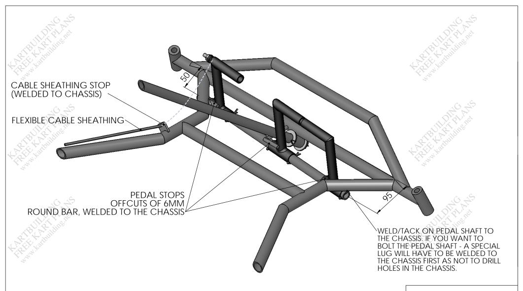
THERE IS A SLIGHT ANGLE BETWEEN THE PEDAL SHAFT AND THE CROSS MEMBERS IN THE CHASSIS. THIS IS BECAUSE THE SEAT IS ANGLED TO ONE SIDE, AND ALLOWS THE DRIVERS FEET REACH ALL THREE PEDALS. THE PEDAL SHAFT CAN BE HELD WITH A VISE-GRIPS/CLAMP TO DETERMINE THE CORRECT DISTANCE AND ANGLE BEFORE WELDING/SECURING THE PEDAL SHAFT TO THE CHASSIS.
