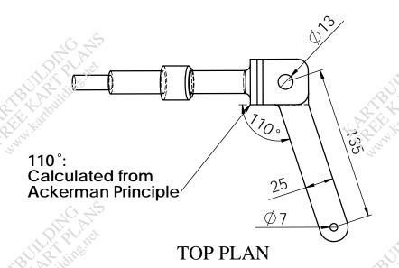
MATERIAL: 6mm FLAT STEEL FOR "n" shape 5mm FLAT STEEL for Steering Arm
