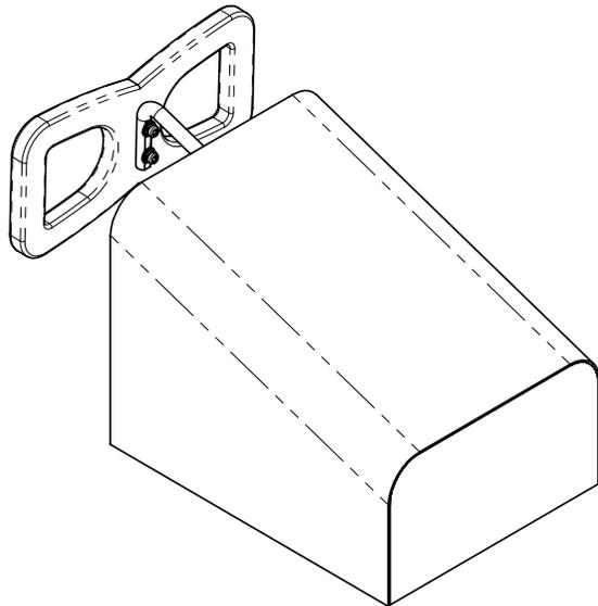
The assembly of the Bonnet is a little tricky. Before the pieces of timber is nailed and glued together, the Steering Column (Steel bar) must be put into position. Once the bonnet assembly is put together, it won't be possible to remove the Steering Column.
