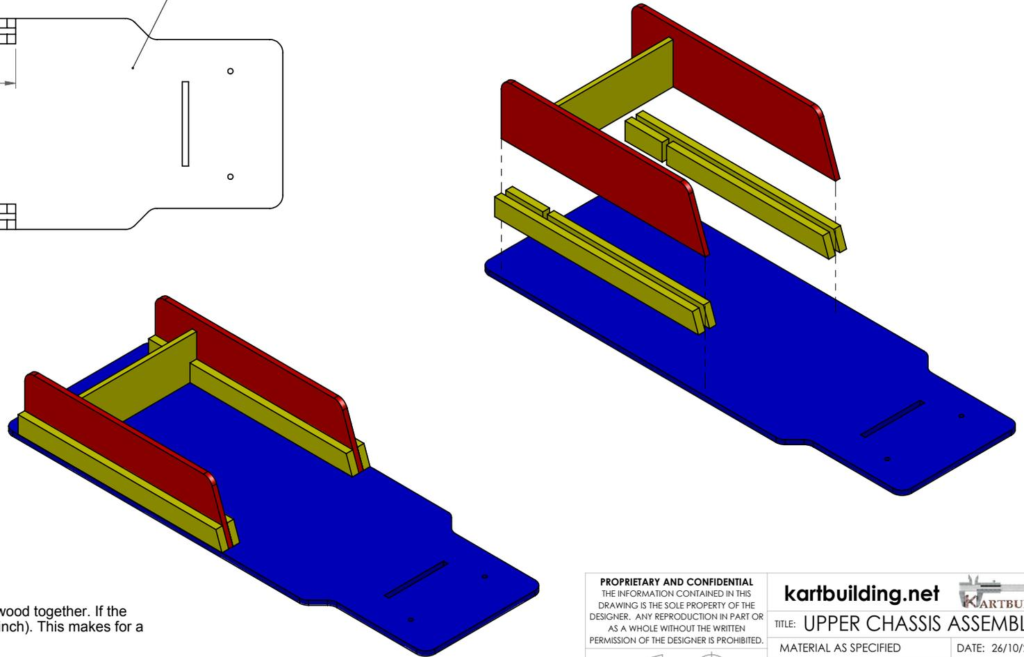
Nails and Wood Glue is used to secure all the pieces of Plywood together. If the nails protrude/stick through, bend the nails back over flat (clinch). This makes for a strong connection.
