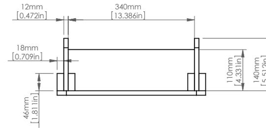
DIMENSIONS FOR THIS IS THE SAME AS ON 'LOWER CHASSIS ASSEMBLY 1' DRAWING
