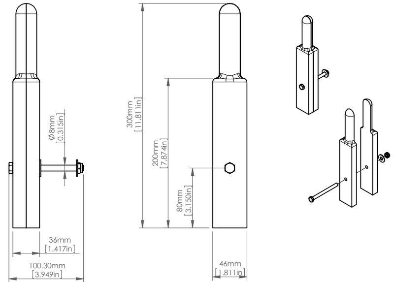
The Brake Lever is to be made from two 18mm [3/4in] thick pieces of timber nailed and glued together. The top of the Lever is to be rounded and shaped as smoothly as possible. Use a wood chisel, file/rasp and sandpaper to shape.
