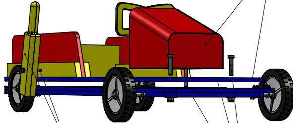
THIRD: Attach the Brake Lever and bolt in place.
