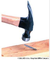
When nailing wood together, the nails should extend and protrude on the other side, where they can be "clinched" and bent over. This makes for a very strong connection.
